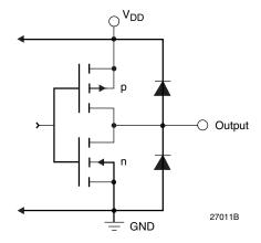
Figure 5. Equivalent Digital Output Circuit
