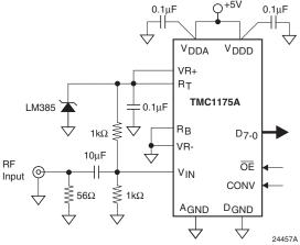
Figure 14. Typical Interface Circuit - Stabilized Reference
