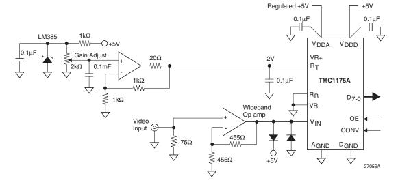
Figure 12. Typical Interface Circuit-High Performance
