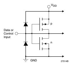
Figure 4. Equivalent Digital Input Circuit
