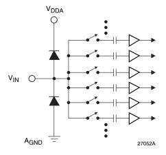
Figure 6. Equivalent Analog Input Circuit
