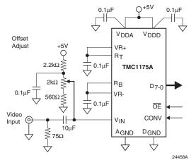
Figure 13. Typical Interface Circuit - Low Cost
