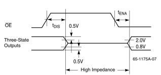
Figure 7. Threshold Levels for Three-State Measurements
