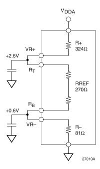
Figure 1. Reference Resistors
